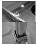
USING 2  $3/8 \times 11/4$ " BOLTS W/ 3/8" SQUARE NUTS, INSERT LEG ASSEMBLY INTO THE 3" X 3" TUBE WITH ROUND SIDE OF LEG FACING TO THE OUTSIDE OF THE FRAME. INSERT BOLTS INTO THE SLOTTED CHANNEL SO THE BOLTS CATCH THE GROVES ON THE BACK SIDE OF THE LEG. THE TOP OF THE LEG SHOULD BE FLUSH WITH THE TOP OF THE 3" X 3" TUBE.
